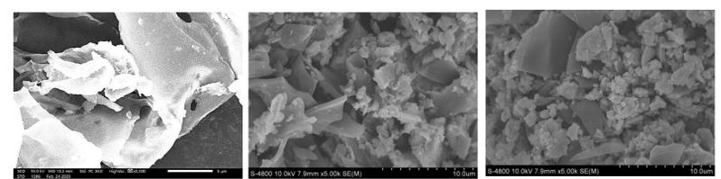
Fig 7. SEM image of AC (A), AC/GO/Fe<sub>3</sub>O<sub>4</sub> before adsorption (B) and AC/GO/Fe<sub>3</sub>O<sub>4</sub> after adsorption (C)
