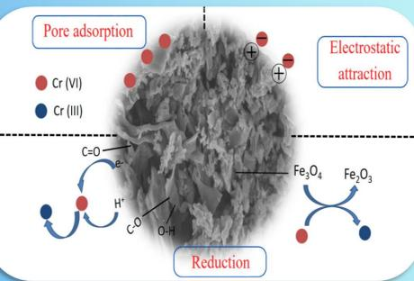
Fig 1. Possible schematic mechanism of Cr (VI) interaction with AC/GO/Fe<sub>3</sub>O<sub>4</sub>
