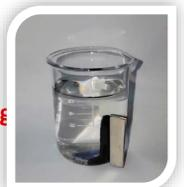
Fig 9. The magnetic of AC/GO/Fe<sub>3</sub>O<sub>4</sub>
