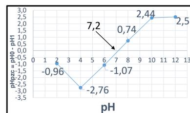
Fig 8. Point of zero charge (pHpzc)
