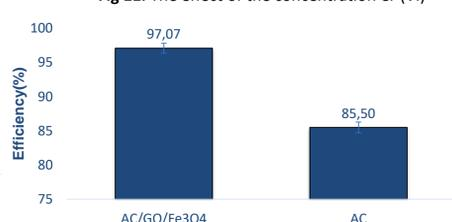
Fig 13. Comparison of Cr (VI) adsorption efficiency between AC/GO/Fe<sub>3</sub>O<sub>4</sub> and AC
