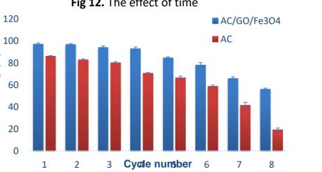
Fig 14. Adsorption efficiency of Cr (VI) over multiple adsorption – desorption cycles
