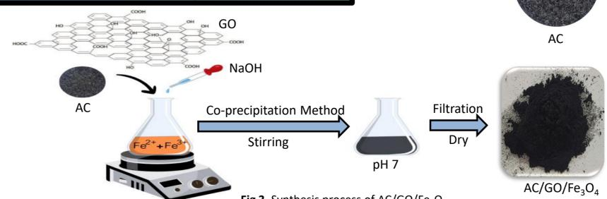
Fig 3. Synthesis process of AC/GO/Fe<sub>3</sub>O<sub>4</sub>
