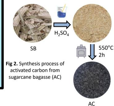
Fig 2. Synthesis process of activated carbon from sugarcane bagasse (AC)
