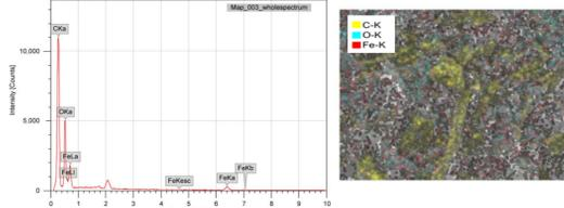
Fig 6. EDX analysis spectrum of AC/GO/Fe<sub>3</sub>O<sub>4</sub>
