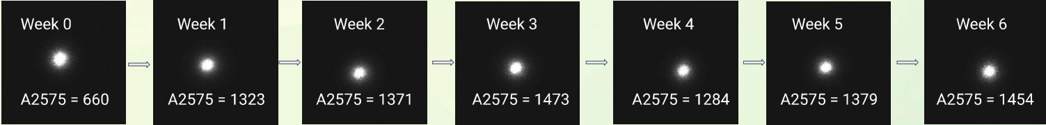
Figure 1. Laser backscattering images and A2575 value of cheese during 6 weeks at 532 nm
