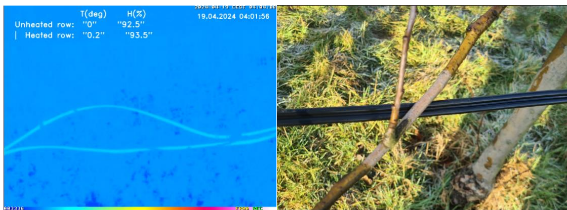
Figure 11: Thermal image of the heating wire captured by MOBOTIX combined with an RGB image
