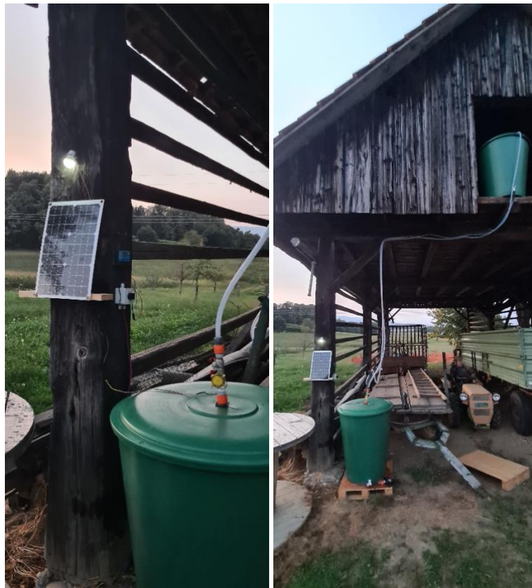
Figure 10: Gravitation battery setup
