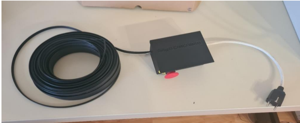
Figure 8: Heating wire system with controller
