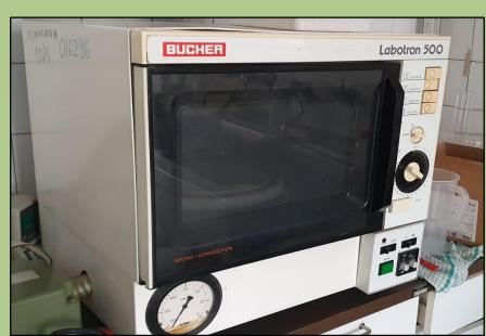
MW irradiation (Labotron 500)
