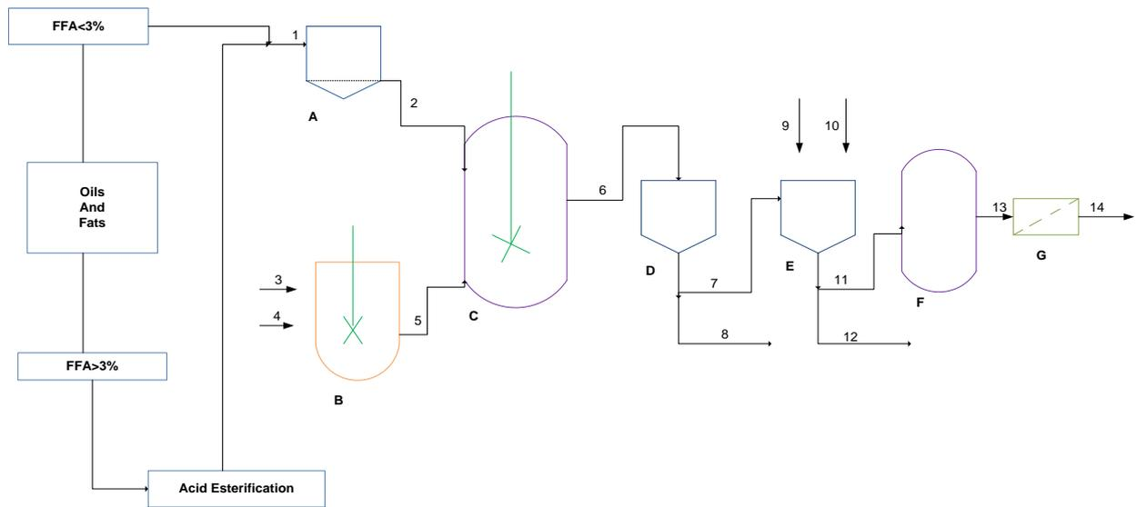
**A:** Filtering and heating tank reactor for Oil and fats
