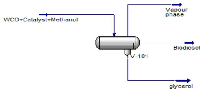
Figure 6 : Separation of Biodiesel and Glycerol
