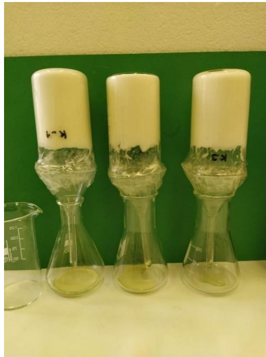
Figure 1.: Measurement setting to determine foam stability
