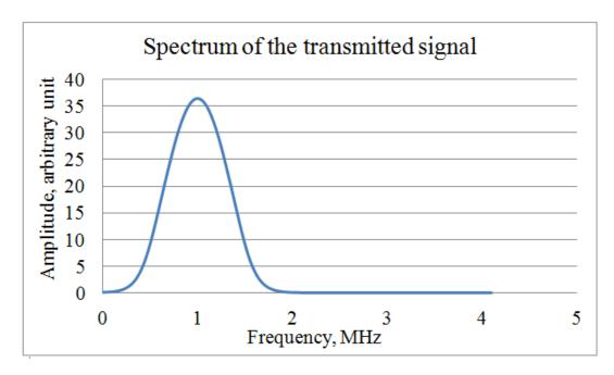
Figure 3: Typical chirp Signal (frequency domain)
