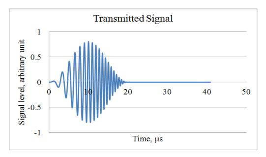
Figure 2. Chirp signal (time domain)
