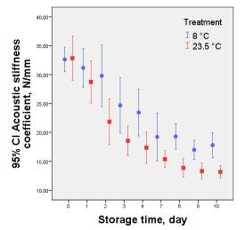
Fig. 3: The changes of the acoustic stiffness coefficient during the storage
