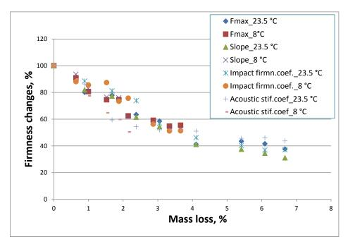
Fig. 6: The percental firmness changes measured by the three different measuring methods vs. mass loss
