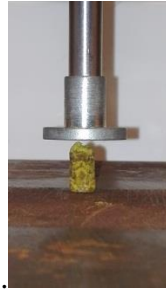
Figure 1 Compression of perga sample between two parallel plates
