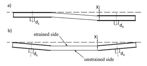
Figure 2: Explanation the adjustment errors of pulleys a) parallel misalignment; b) angular misalignment
