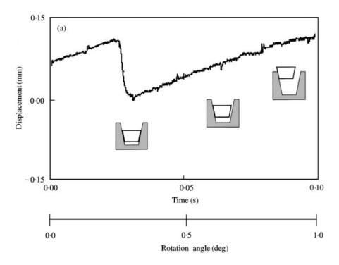
Figure 1: Stick-slip behaviour of V-belt in the groove
