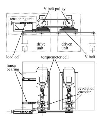
Figure 3: The structure of the test equipment
