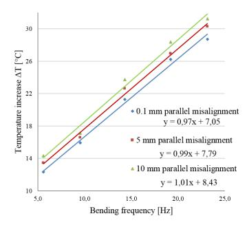
Figure 5: The heat generated as a consequence of the parallel misalignment of V-belt pulleys as a function of bending frequency
