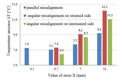
Figure 6: The temperature increase of the V-belt drive due to geometrical adjustment errors as a function of the extent of the error
